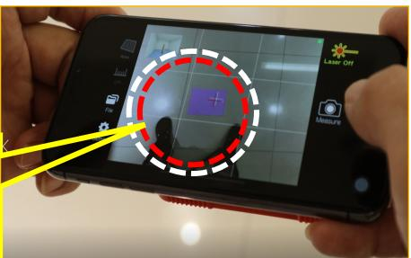
4.3 Tilt the angle back and forth slightly holding your camera, the red cross should be adjusted to overlap with the white cross, and a GREEN cross will appear on the screen once aligned. If not, the adjustment icon as shown here will appear when trying to click "measure".
